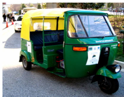
The Indian Bajaj three-wheeler single-cylinder i.c. engine taxi converted by Energy Conversion Devices from CNG to metal hydride fuel.
